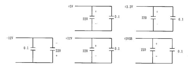
0.1uf is ceramic the other is electrolytic capacitor.
